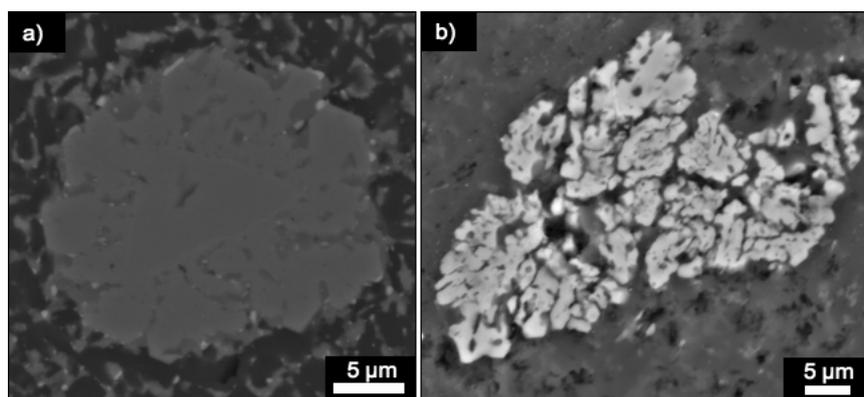
Fig. 1 - New garnet in the pseudotachylyte matrix. a) Dendritic overgrowth of new garnet around a small clast of granulitic garnet within the pseudotachylytes inside metagabbro. The pseudotachylytes matrix is composed by labradorite-bytownite plagioclase (77.5%), orthopyroxene (11.8%) and dispersed ore mineral. BSE-SEM image. b) Dendritic garnet in the pseudotachylytes within the kinzigite-mylonites. The matrix is composed by quartz, oligoclase, K-feldspar and biotite. BSE-SEM image.
